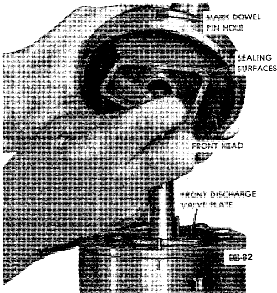
Figure 9B-108 Placing Front Head on Cylinder Assembly - 6 Cylinder Compressor
