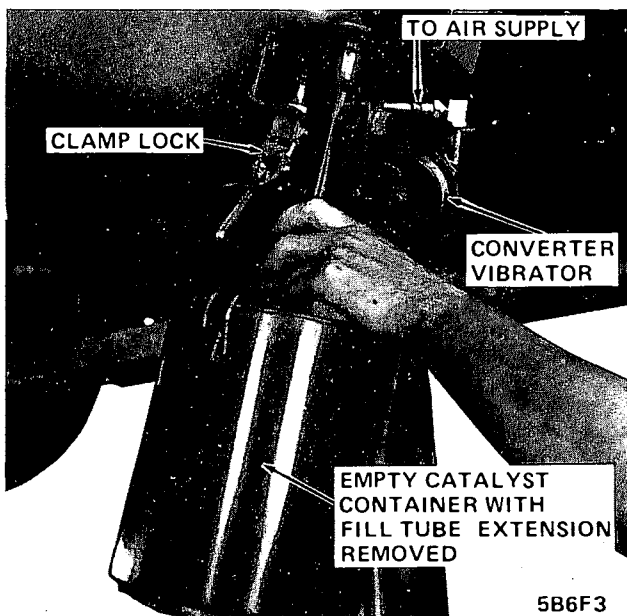
Figure 6F-8 - Clamping on Vibrator and Empty Catalyst Container
