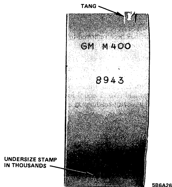
Figure 6A-73 - Location of Undersize Mark on Bearing Shell
