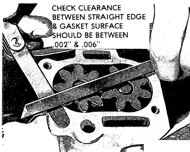
Figure 6A-104 - Checking Oil Pump End Clearance
