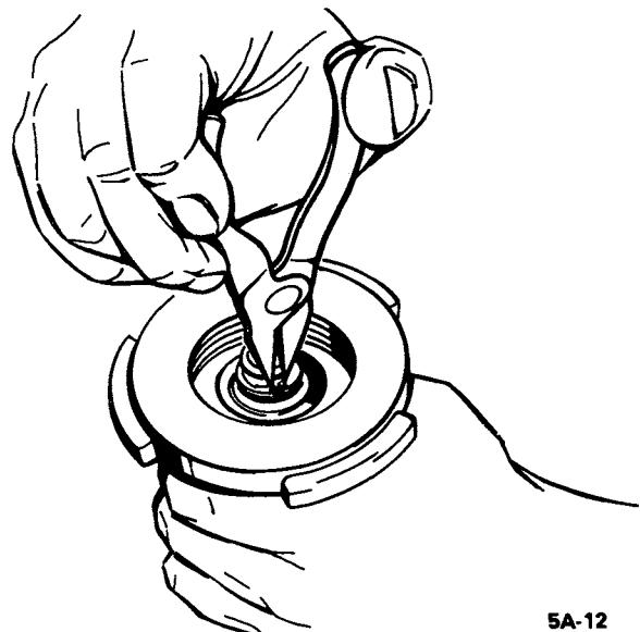
Figure 5A-13 Removing Retaining Ring From Air Valve
