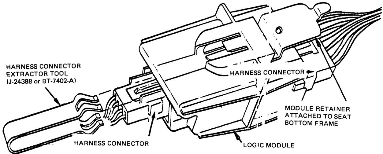
Figure 1B-11 Removing Connectors from Module
