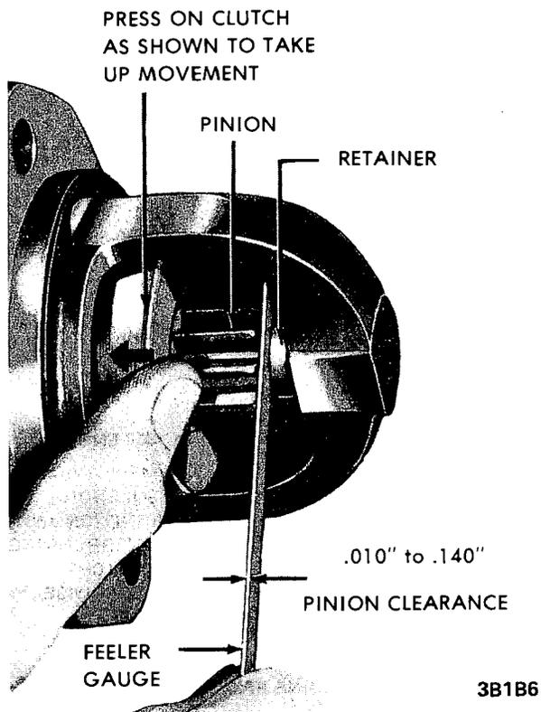
Figure 1B-6 Checking Pinion Clearance
