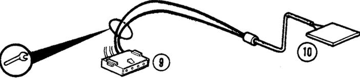
REPAIR OPEN CIRCUIT IN ONE OR BOTH WIRES FROM 4-WIRE CONN. TO SEAT SENSOR CONN.</p>                                                                                                                                                                                                           | <p>
