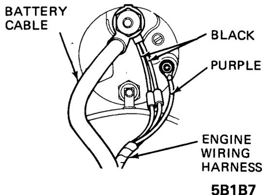
Figure 1B-7 Typical Solenoid Wire Connection
