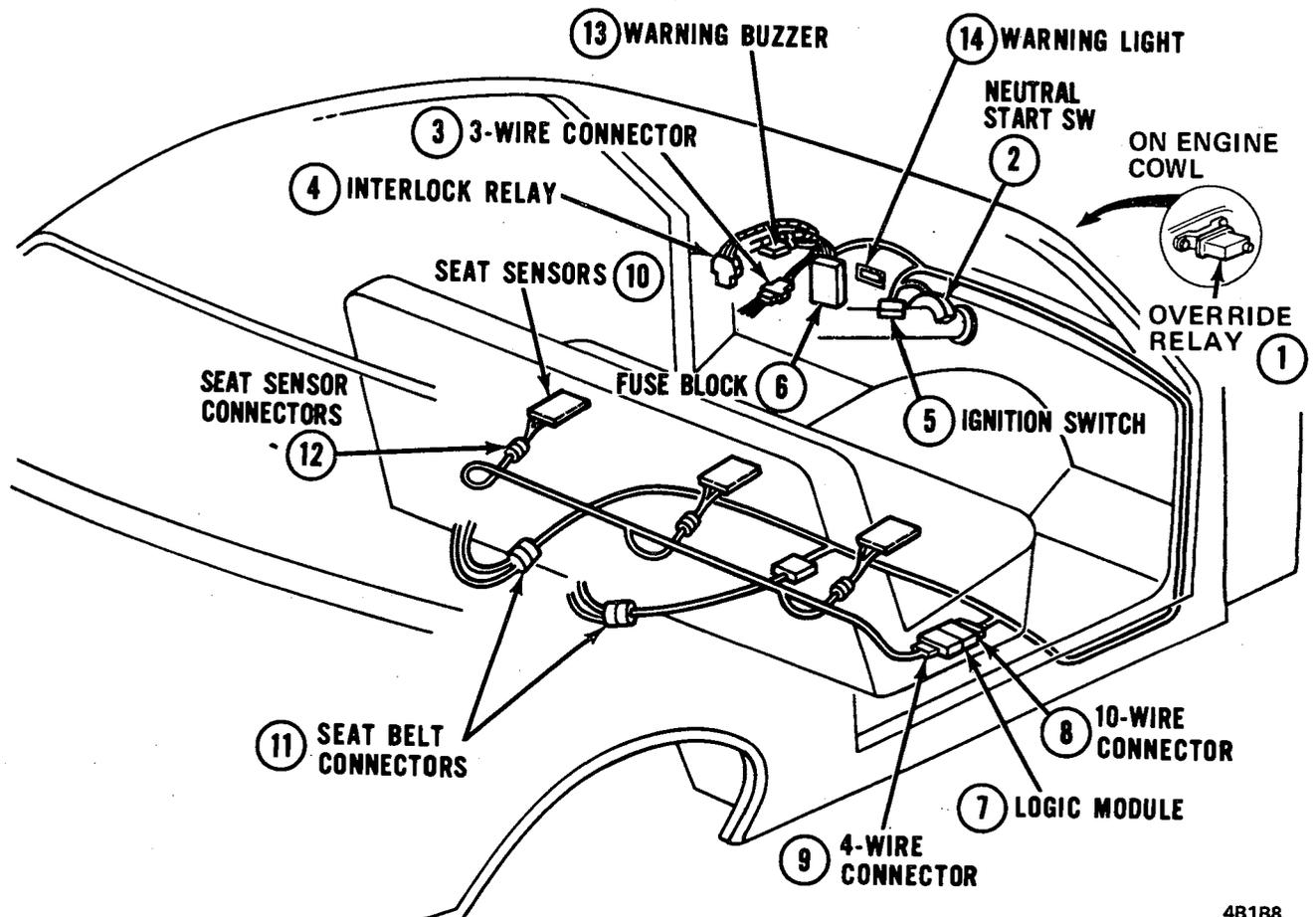
Figure 1B-8 System Components and location
