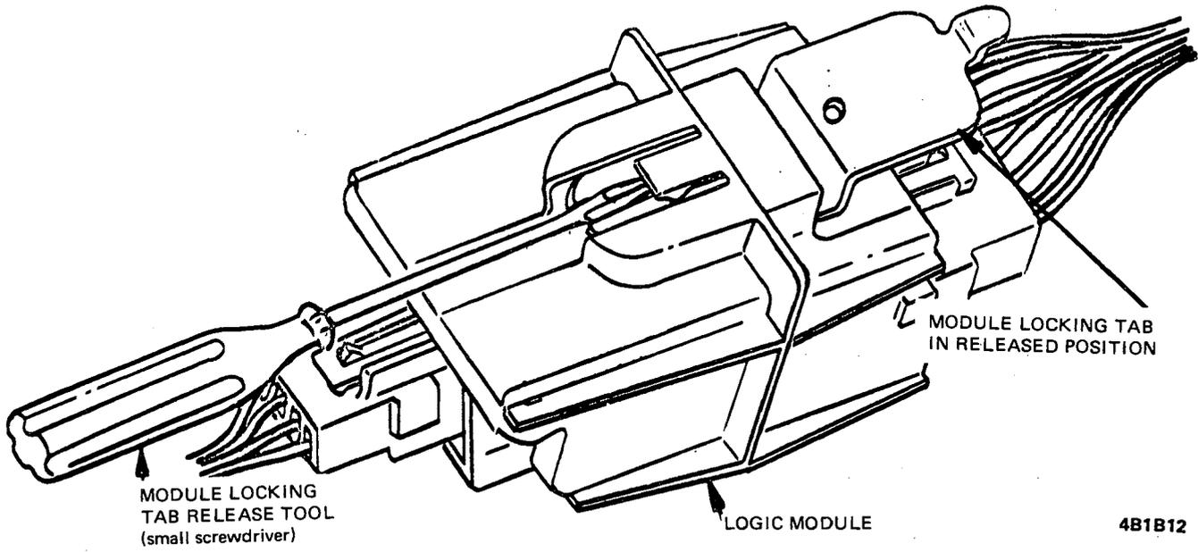
Figure 1B-12 Removing Module from Retaining Bracket
