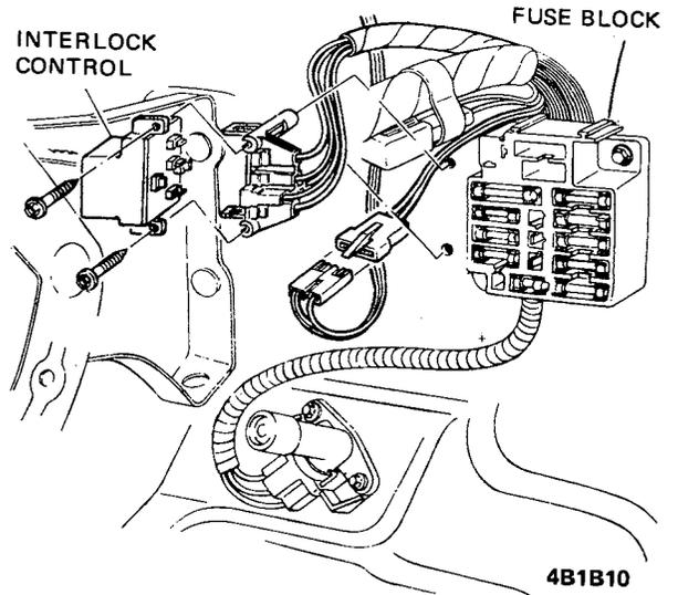
Figure 1B-10 Interlock Relay Removal (B-C-E Shown)
