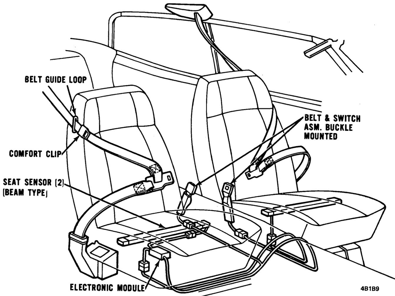
Figure 1B-9 Beam Type Seat Sensor Installation
