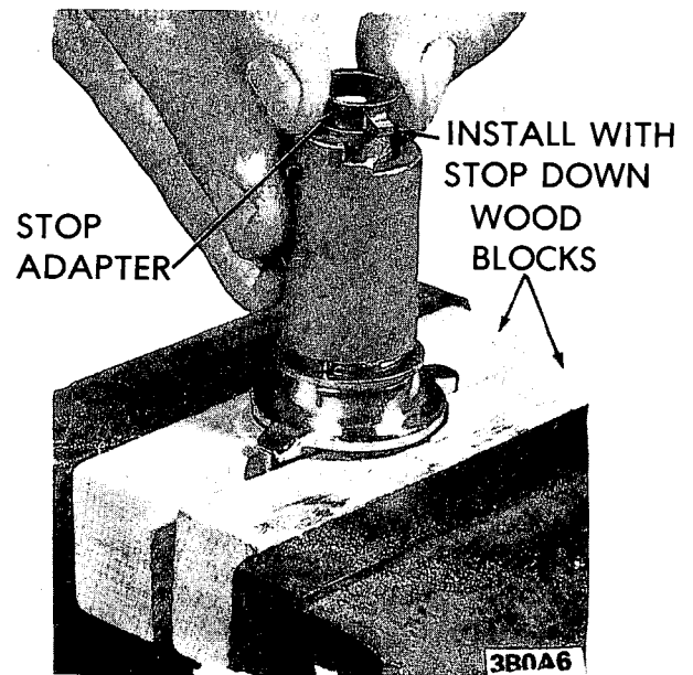
Figure OA-6 Installing Stop Adapter on Lock Cylinder
