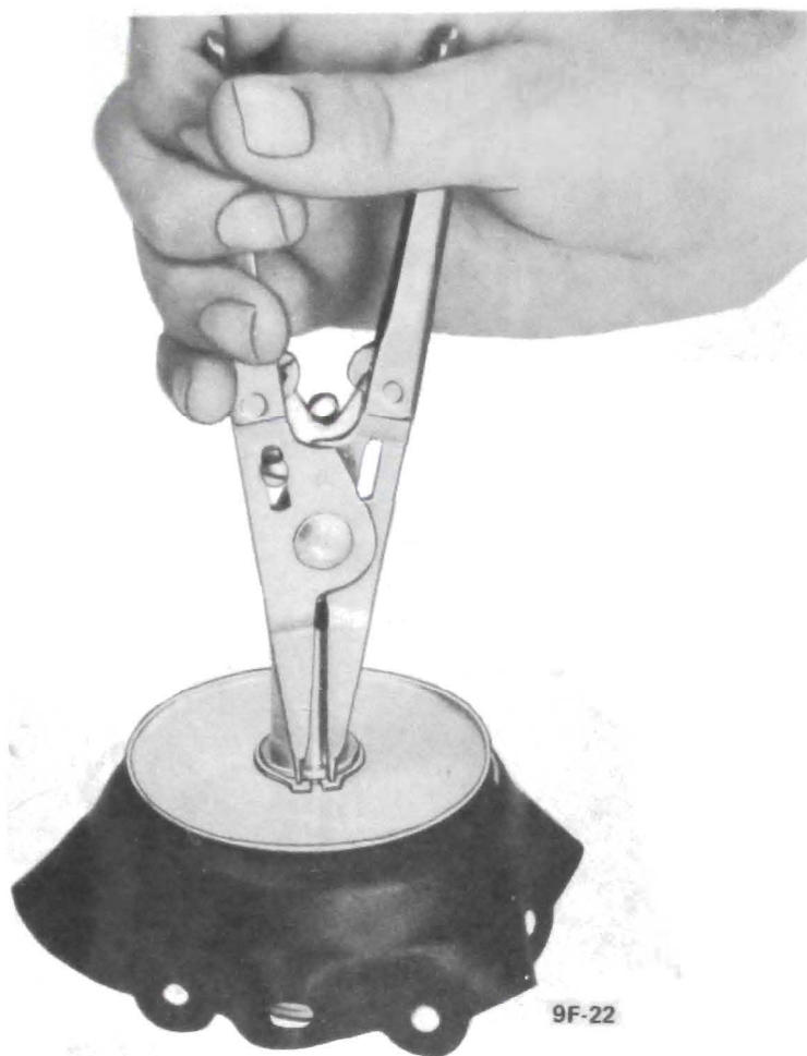
Figure 9F-11 - Removing Snap Ring
