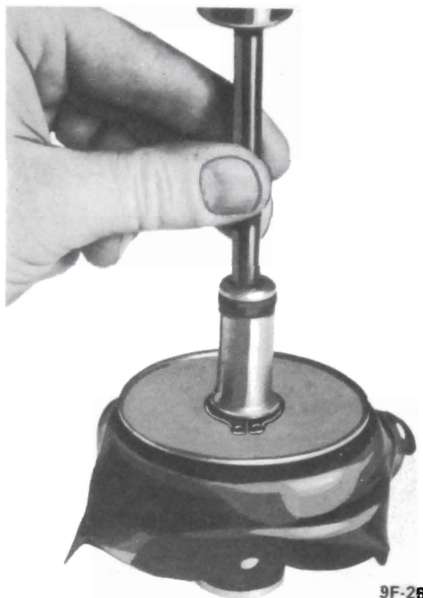
Figure 9F-15 - Installing Check Valve
