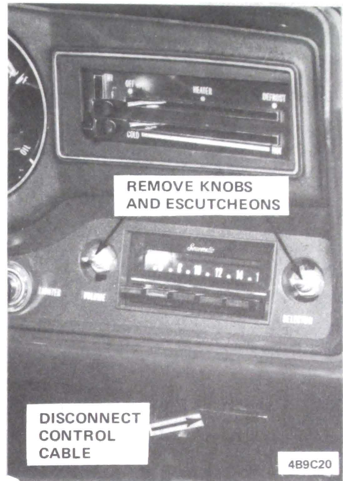
Figure 9C-23 Center Air Duct Control
