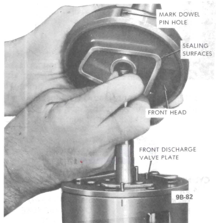
Figure 9B-96 Placing Front Head on Cylinder Assembly
