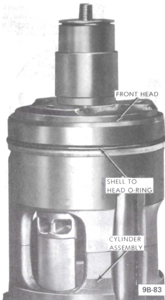
Figure 9B-97 Shell to Front Head O Ring Installation
