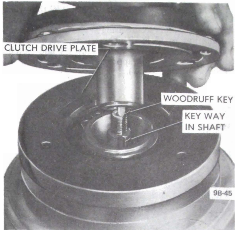
Figure 9B-52 Positioning Clutch Drive Plate on Shaft
