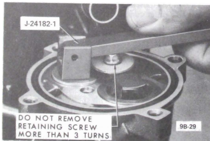
Figure 9B-33 Capsule Removal Tool Attached to TX Valve Capsule
