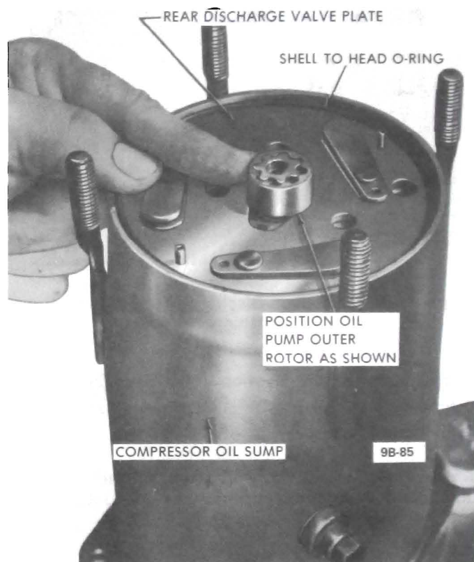
Figure 9B-100 Positioning Oil Pump Outer Rotor
