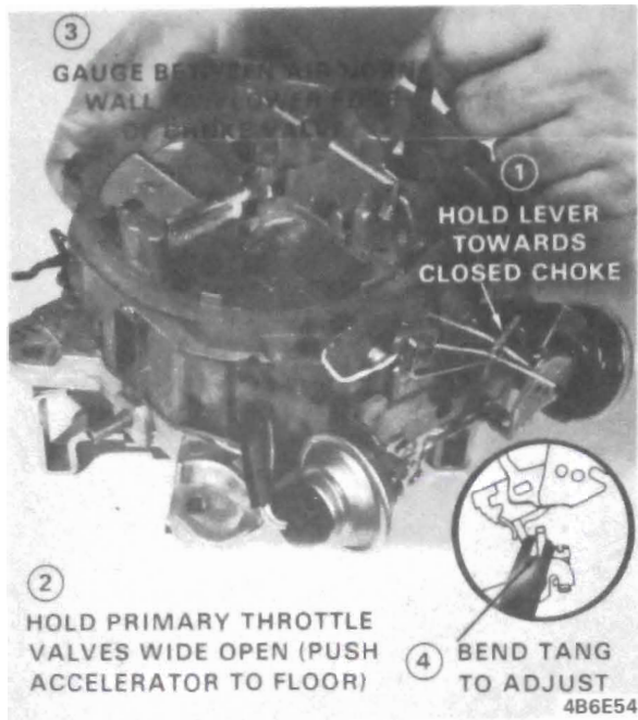
Figure 6E-54 Choke Unloader Adjustment
