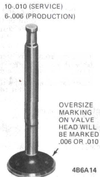
Figure 6A-63 - Oversize Valve Identification
