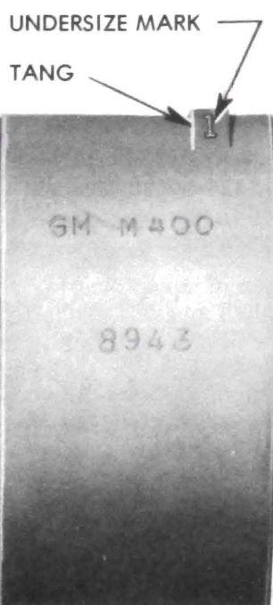
Figure 6A-75 - Location of Undersize Mark on Bearing Shell
