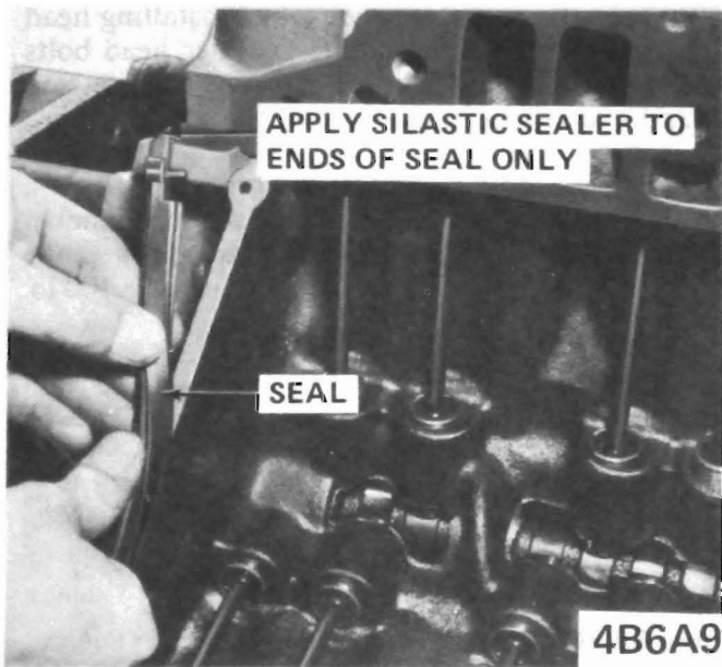
Figure 6A-58 - Intake Manifold Seal Installation
