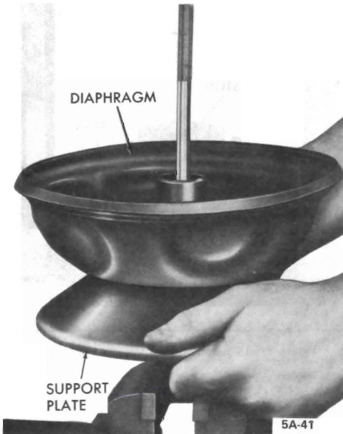
Figure 5A-41 Positioning Power Piston on Support Plate Remover
