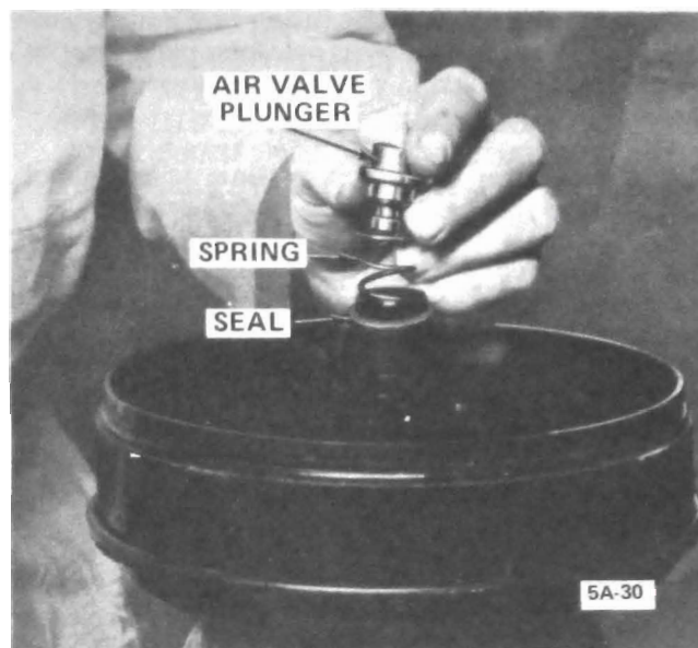
Figure 5A-30 Installing Air Valve Plunger
