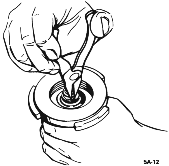
Figure 5A-13 Removing Retaining Ring From Air Valve
