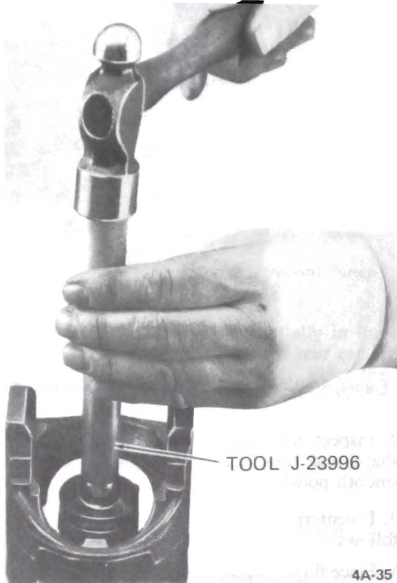
Figure 4A-35 Installing Ball Using Tool J-23996
