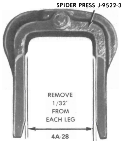
Figure 4A-28 Spider Press Leg Rework
