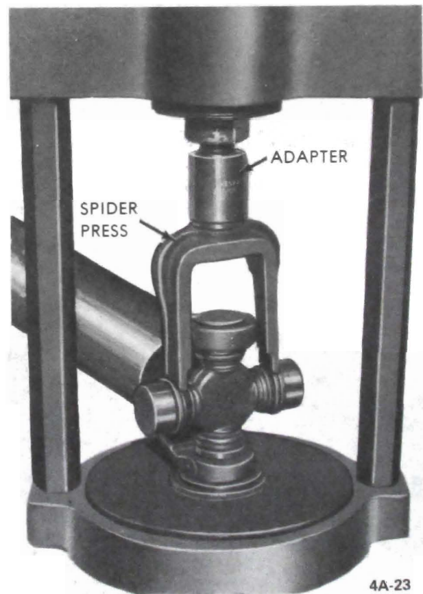
Figure 4A-23 - Pressing Out U-Joint Bearing
