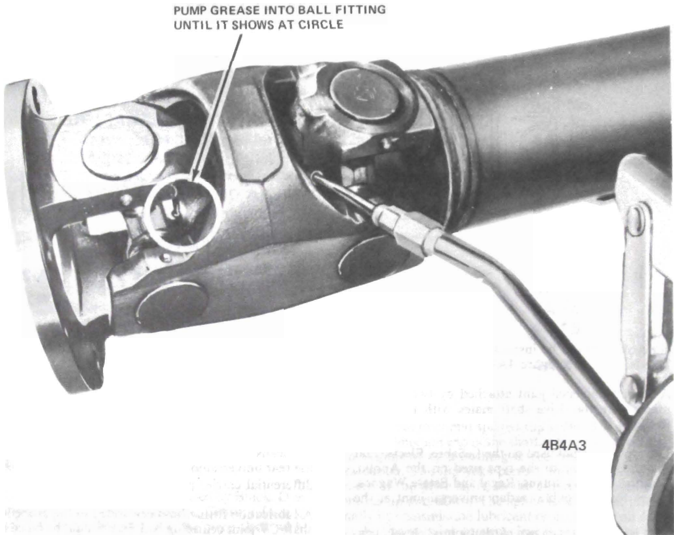
Figure 4A-4 CV Joint Centering Ball Lube Fitting
