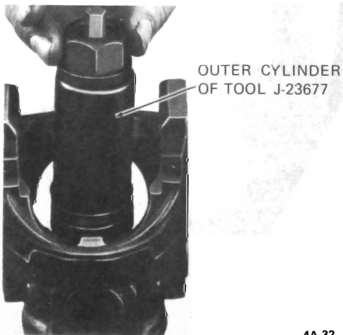
Figure 4A-32 Second Step - Removing Centering Ball with Tool J-23677
