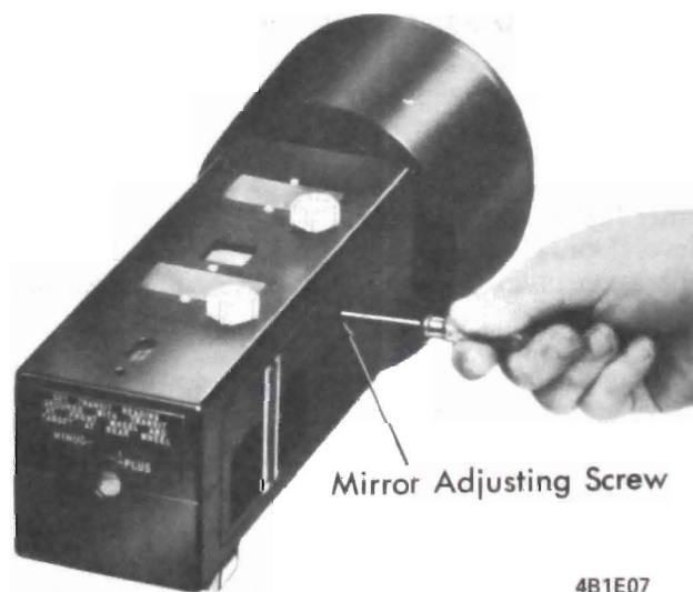
Figure 1E-5 Adjusting Horizontal Calibration
