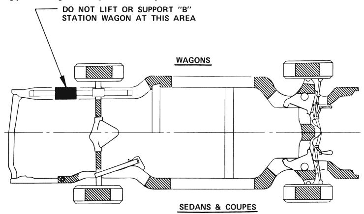
NOTE: SUPPORTS MUST BE POSITIONED SO AS TO DISTRIBUTE LOAD AND SUPPORT VEHICLE IN A STABLE MANNER
