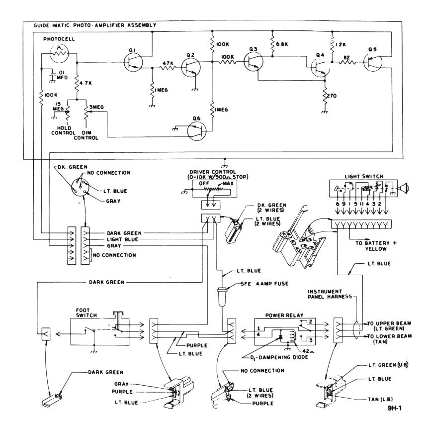
Figure 9H-1 Guide-Matic Schematic
