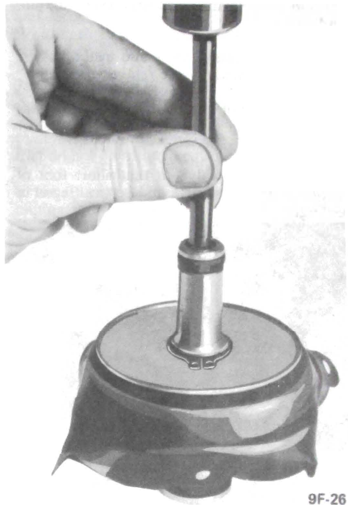
Figure 9F-35 - Installing Check Valve
