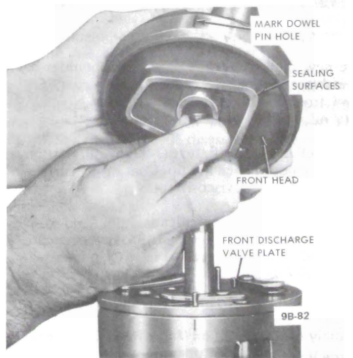
Figure 9B-82 Placing Front Head on Cylinder Assembly
