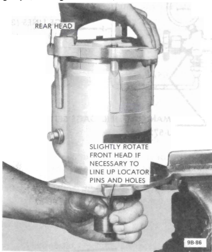
Figure 9B-101 Installing Rear Head
