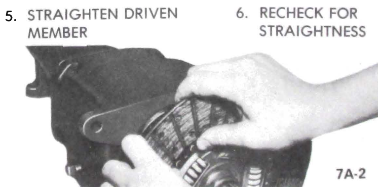
Figure 7A-2 - Checking Driven Plate Run-Out
