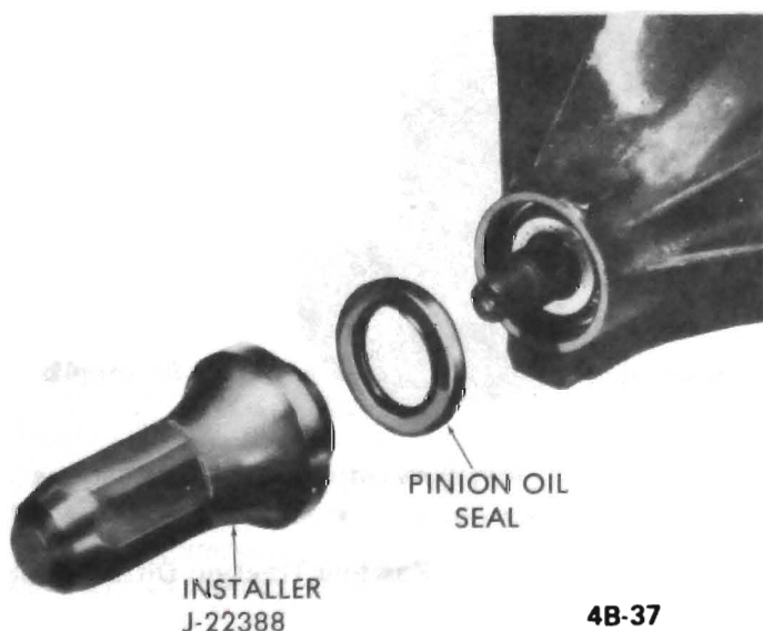
Figure 4B-37 - Installing Pinion Oil Seal
