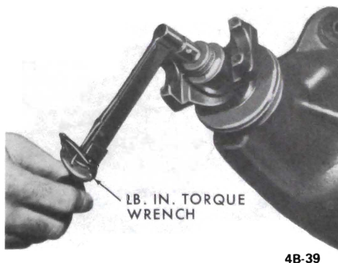
Figure 4B-39 - Checking Pinion Preload
