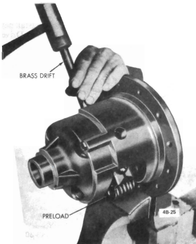
Figure 4B-25 Removing Preload Thrust Blocks and Springs
