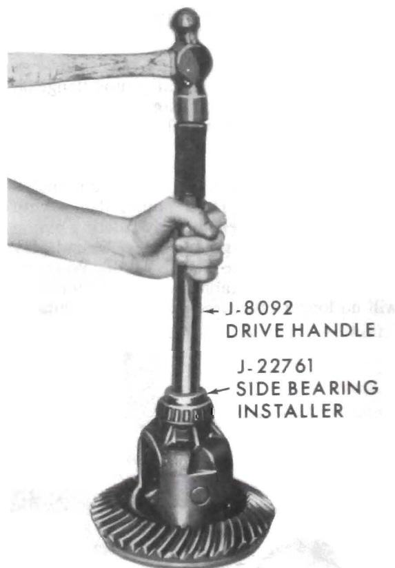
Figure 4B-41 - Installing Differential Side Bearings
