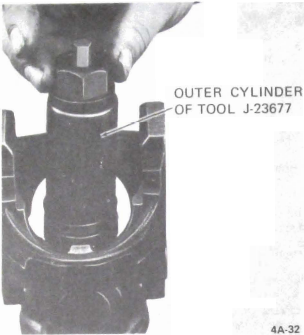
Figure 4A-32 Second Step - Removing Centering Ball with Tool J-23677
