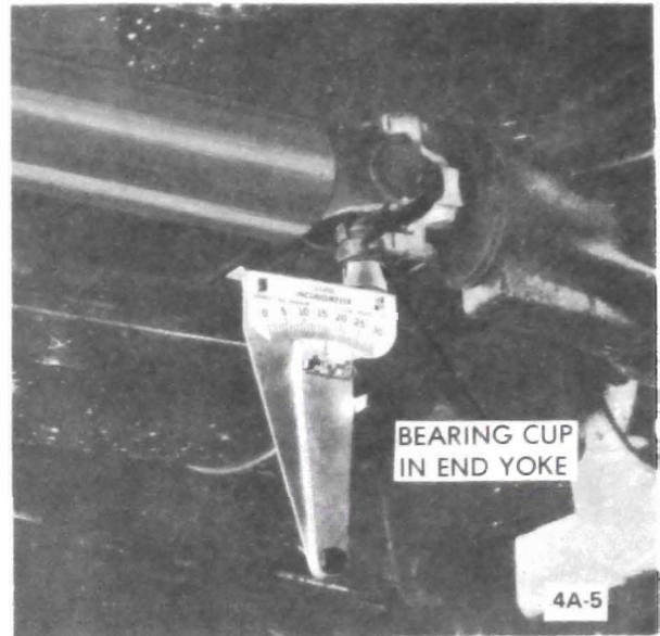
Figure 4A-5 Measuring Angle at Rear of Propeller Shaft
