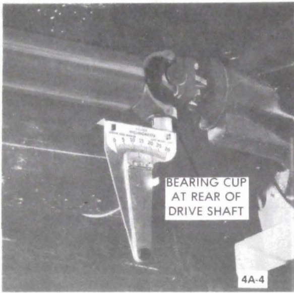
Figure 4A-4 Measuring Angle at Rear of Propeller Shaft
