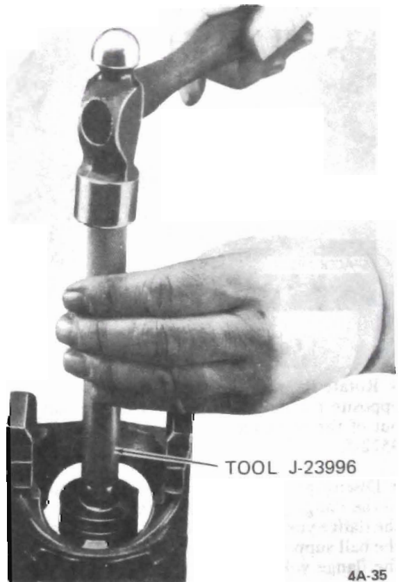
Figure 4A-35 Installing Ball Using Tool J-23996
