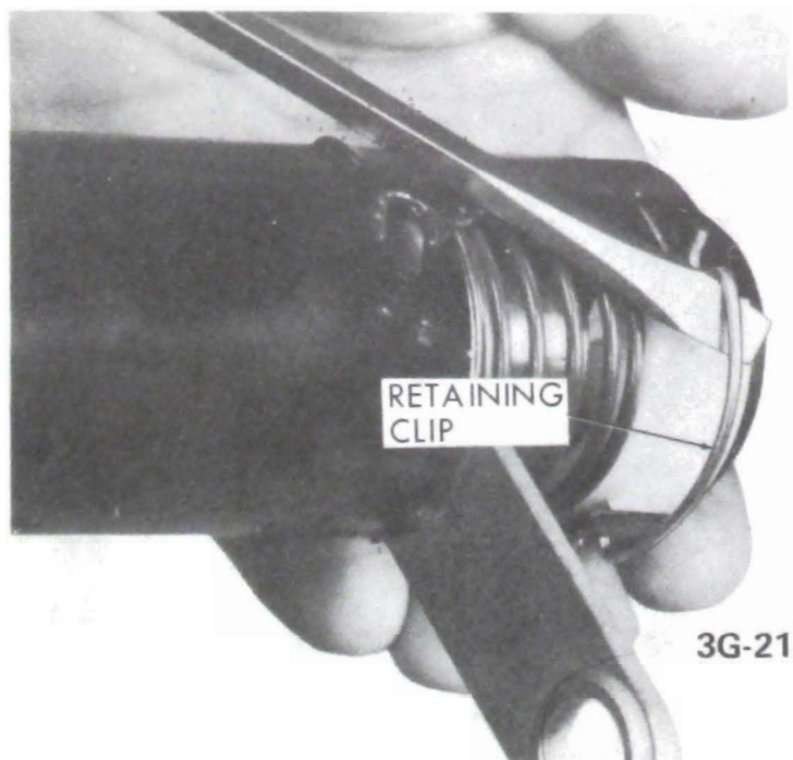
Figure 3G-21 Removing Bearing Adapter Clip
