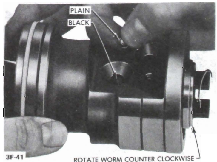
Figure 3F-41 Loading Balls in Rack-Piston Nut
