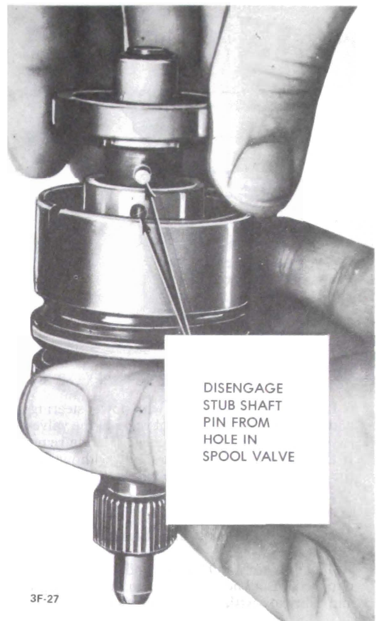
Figure 3F-27 Removing Stub Shaft Assembly
