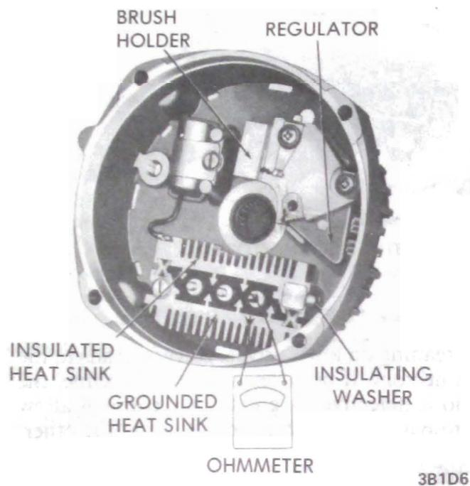
Figure 1D-6 Checking Rectifier Bridge
