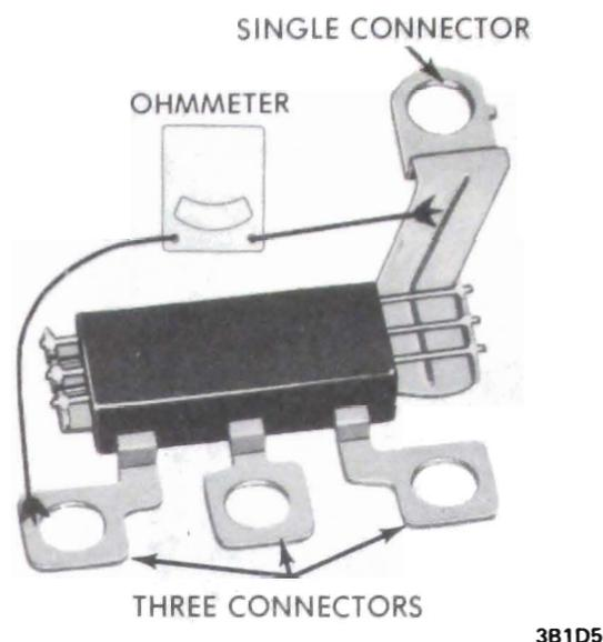
Figure 1D-5 Checking Diode Trio
