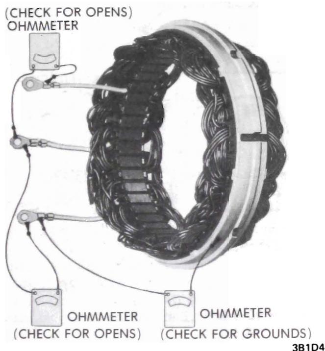
Figure 1D-4 Checking Stator Windings
