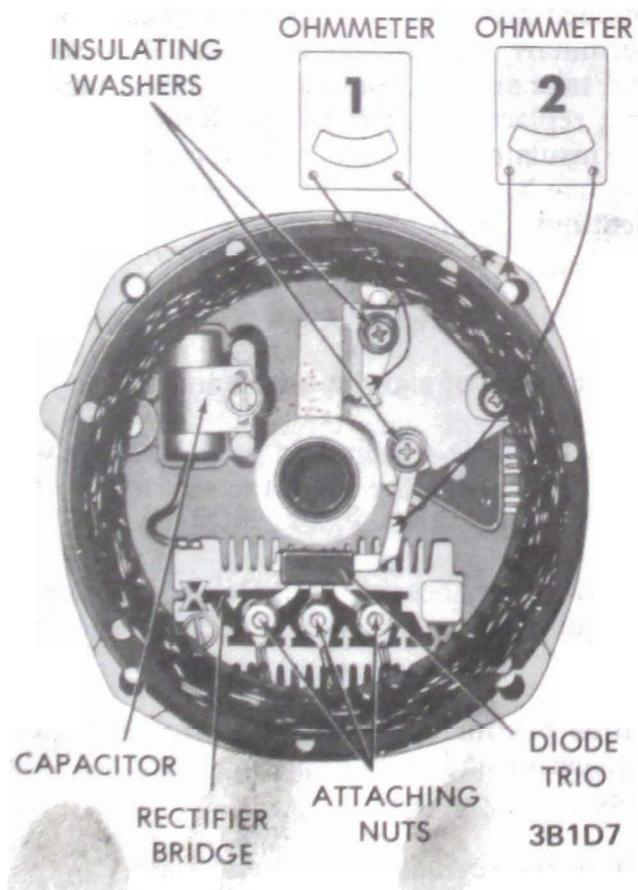
Figure 1D-7 Checking Diode Trio
