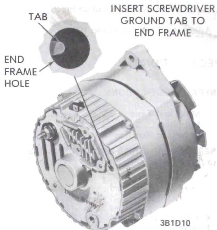
Figure 1D-10 Grounding Field Windings
