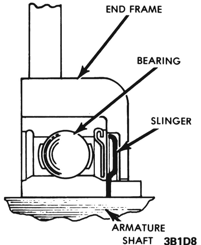
Figure 1D-8 Drive End Bearing Assembly
