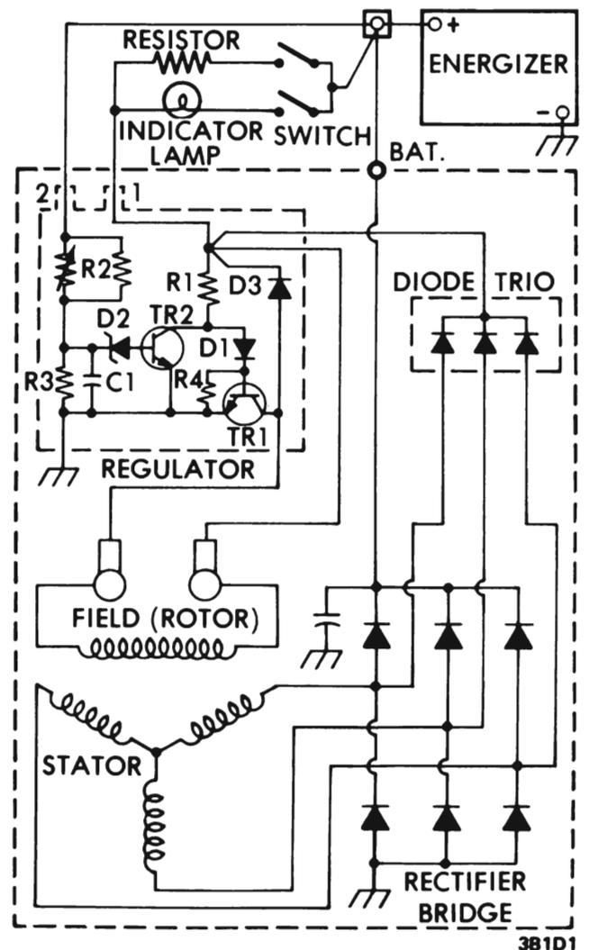
Figure 1D-1 Delcotron Wiring Schematic
