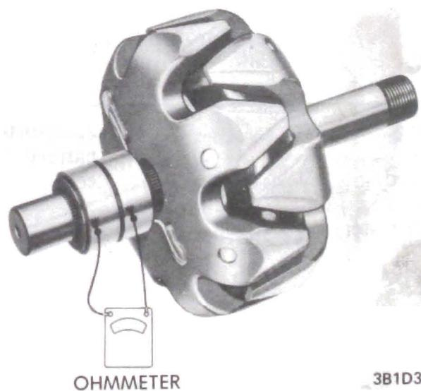
Figure 1D-3 Checking Rotor for Opens and Shorts
