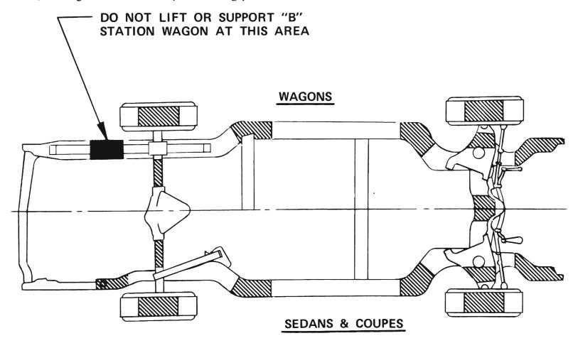
NOTE: SUPPORTS MUST BE POSITIONED SO AS TO DISTRIBUTE LOAD AND SUPPORT VEHICLE IN A STABLE MANNER
