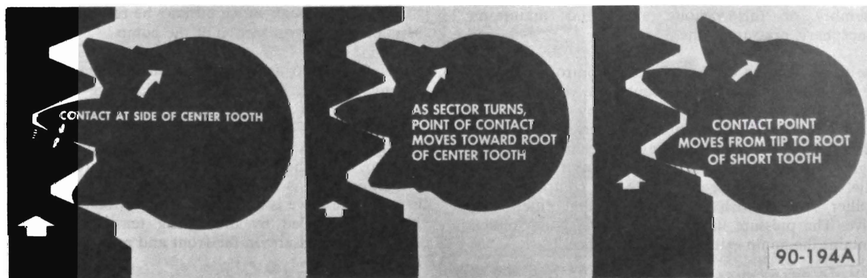
Figure 90-23 - Steering Gear Tooth Contact
