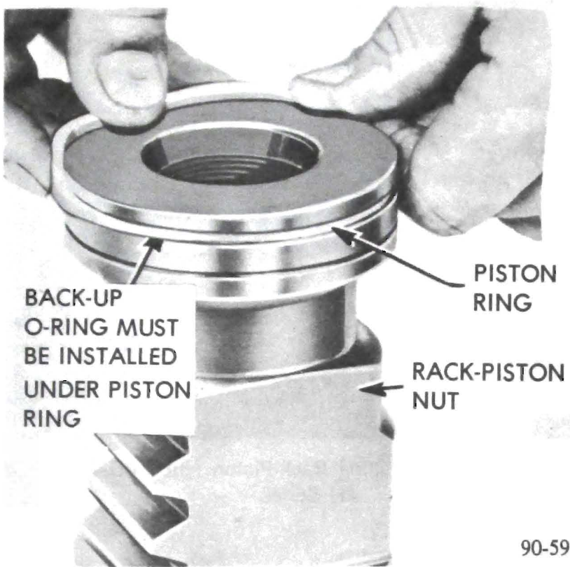
Figure 90-59 Installing Rack-Piston Ring on Rack-Piston Nut
