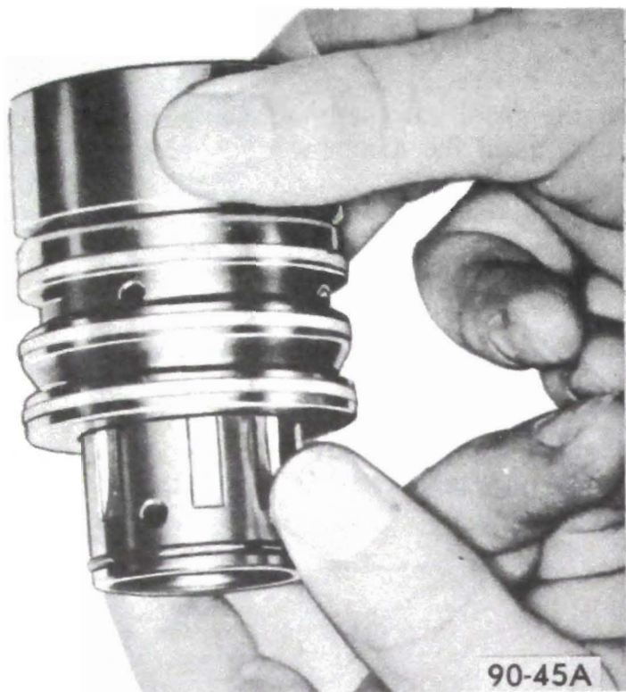
Figure 90-45 Removing Spool Valve
