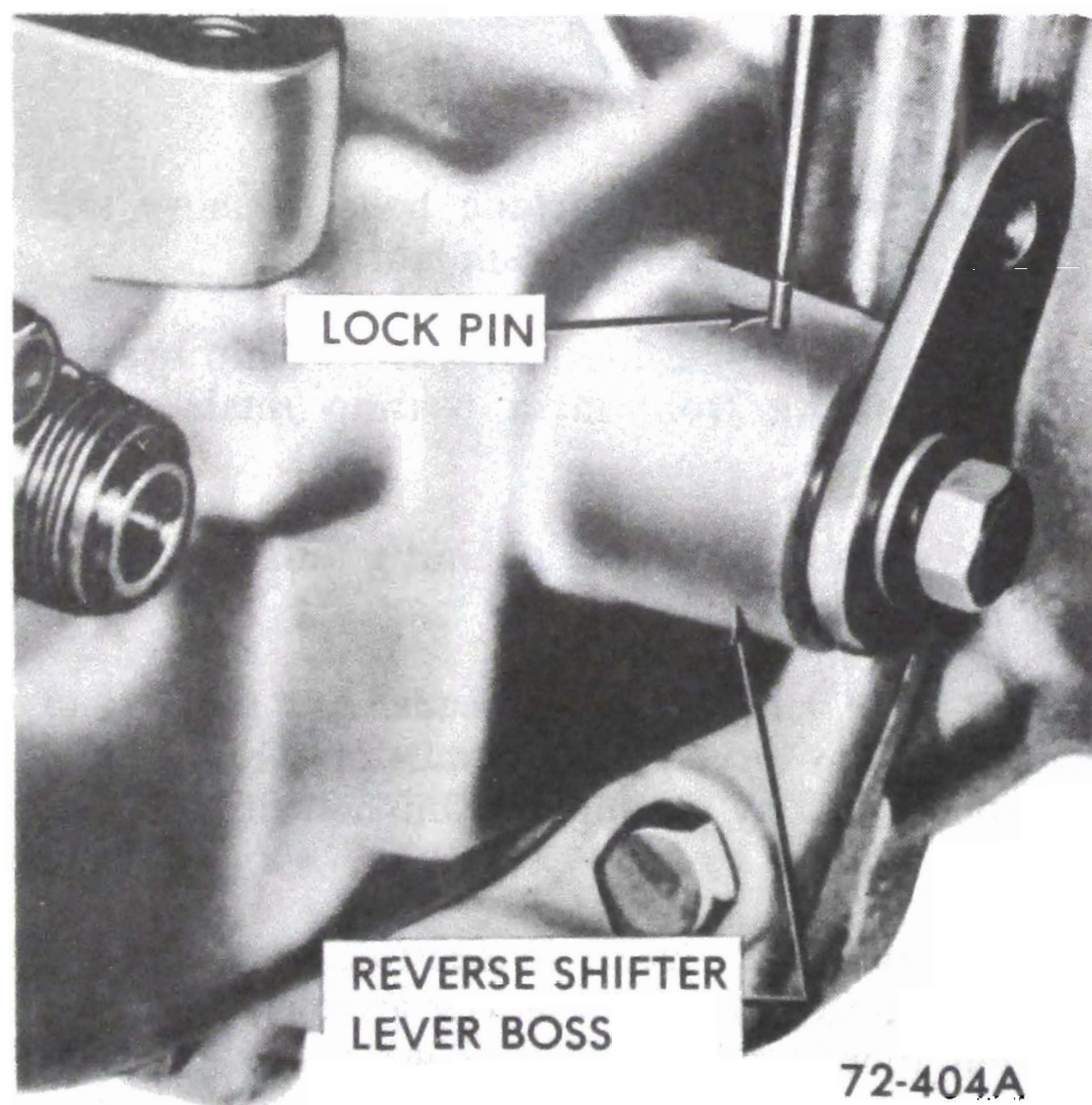
Figure 72-41 - Removing Shifter Shaft Lock Pin
