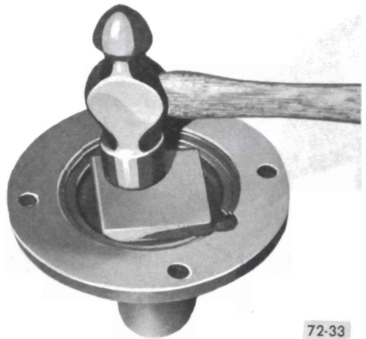
Figure 72-31 - Installing Front Bearing Retainer Seal
