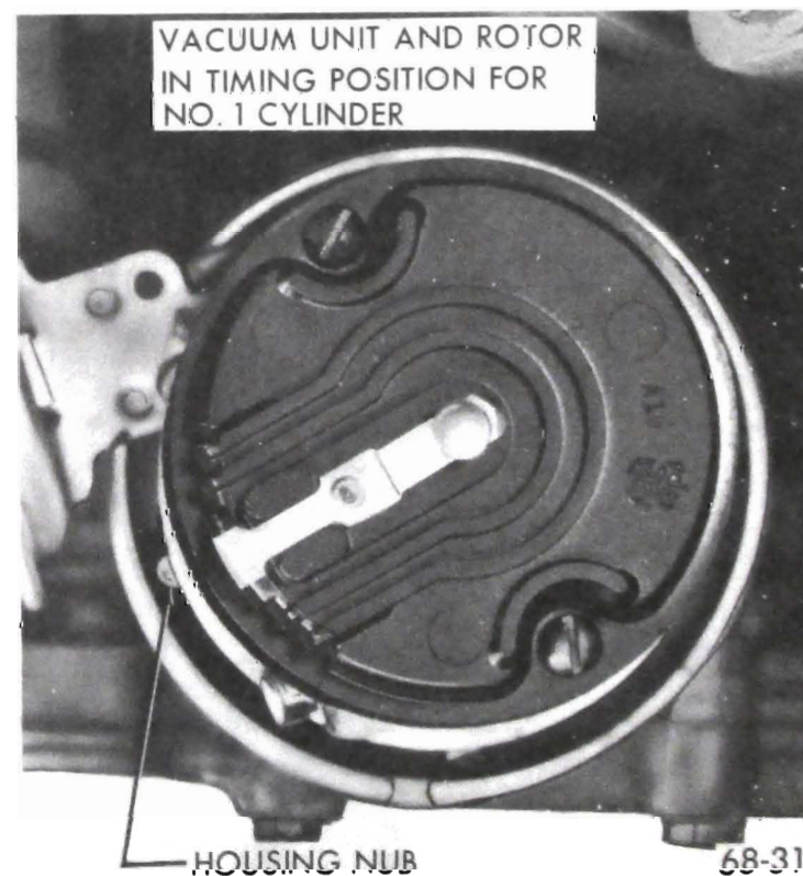
Figure 68-28 - Installing Distributor in Engine
