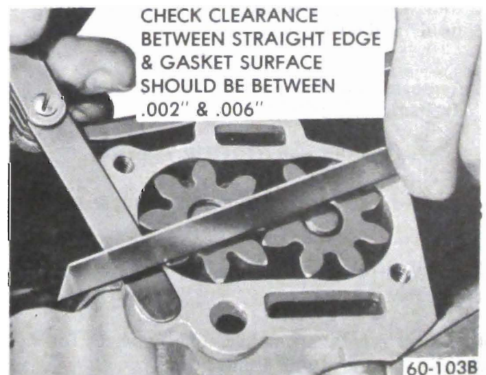
Figure 60-59 - Checking Oil Pump End Clearance
