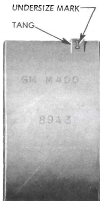
Figure 60-33 - Location of Undersize Mark on Bearing Shell
