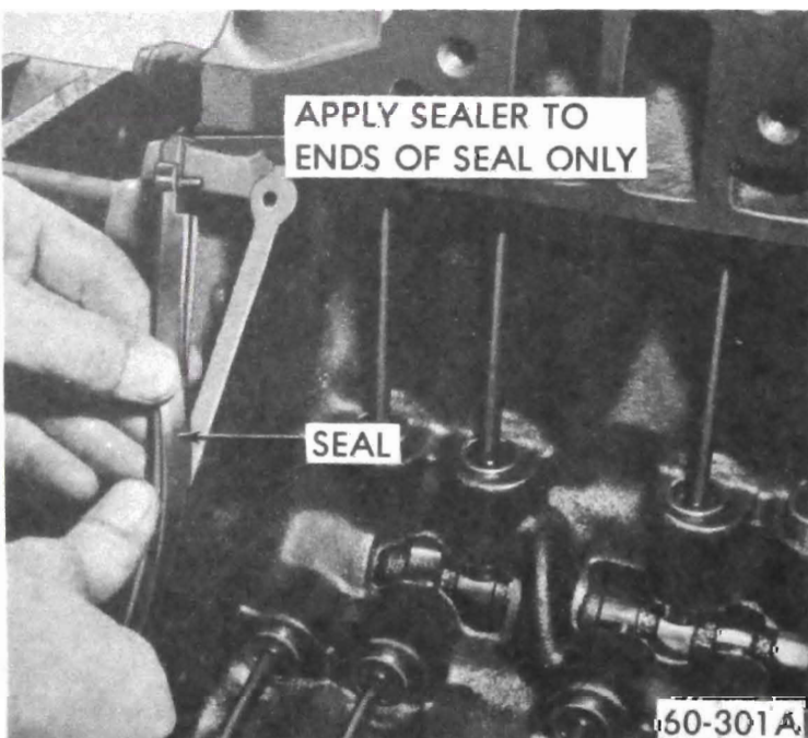
Figure 60-15 - Intake Manifold Seal Installation
