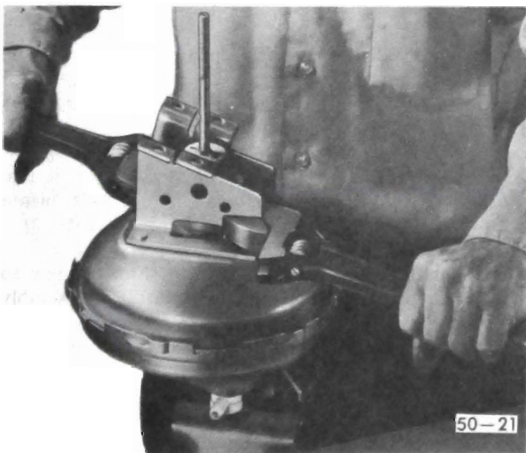
Figure 50-101 Separating Power Brake Unit-4D-4F-4G-4H
