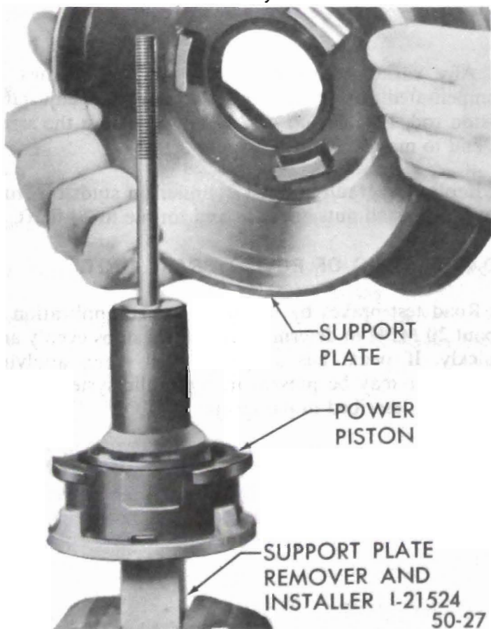
Figure 50-113 Installing Power Piston into Support Plate
