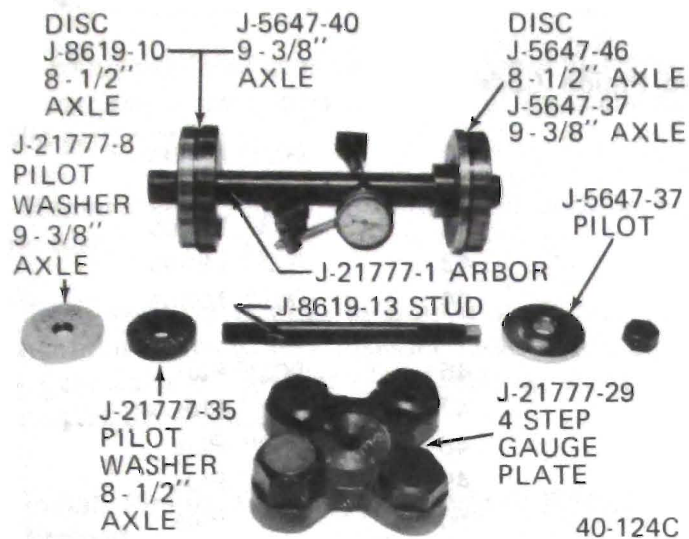
Figure 40-129 - Pinion Setting Gauge
