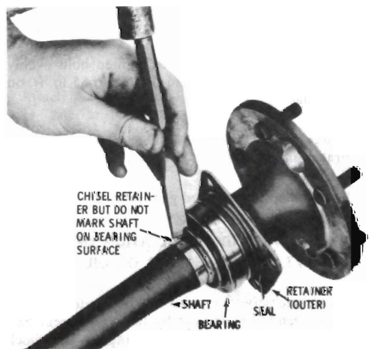
Figure 40-113 - Removing Axle Shaft Bearing Retainer
