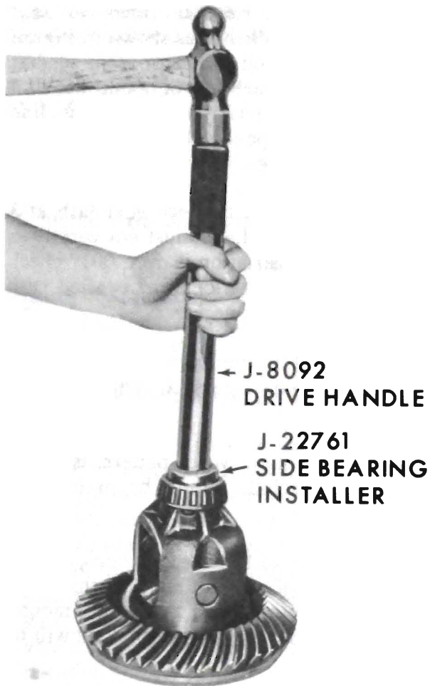
Figure 40-138 - Installing Differential Side Bearings
