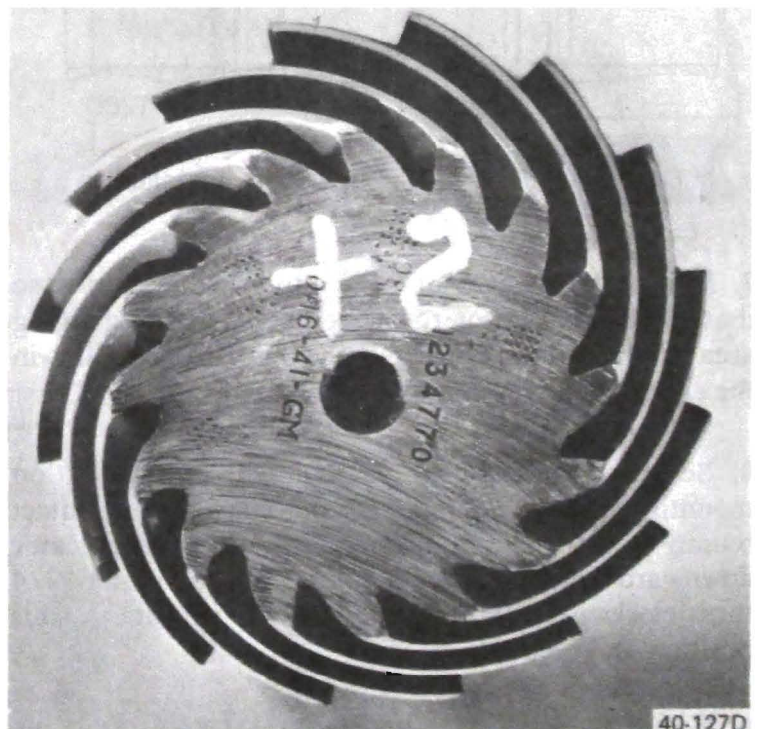
Figure 40-132B Pinion Marking "B" Type Axle
