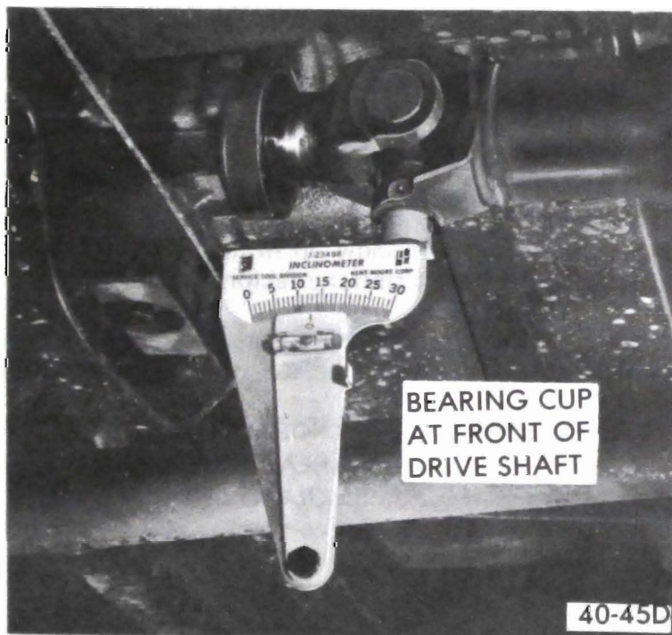
Figure 40-54 Measuring Angle at Front or Propeller Shaft
