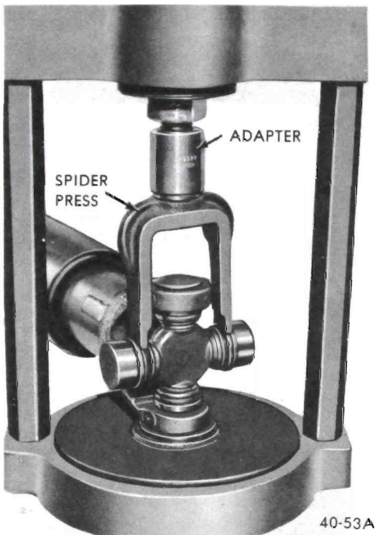
Figure 40-60 - Pressing Out U-Joint Bearing
