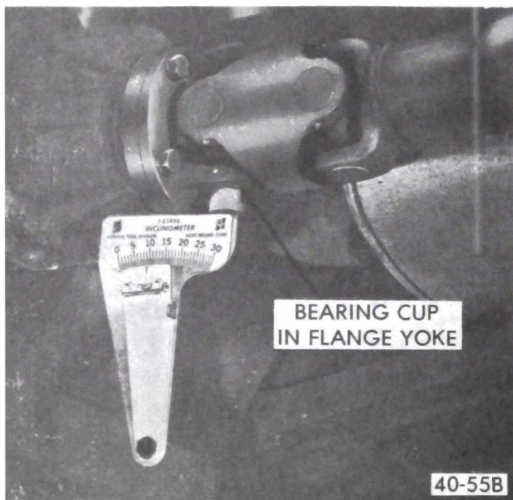
Figure 40-55B - Measuring Angle at Rear of Propeller Shaft
