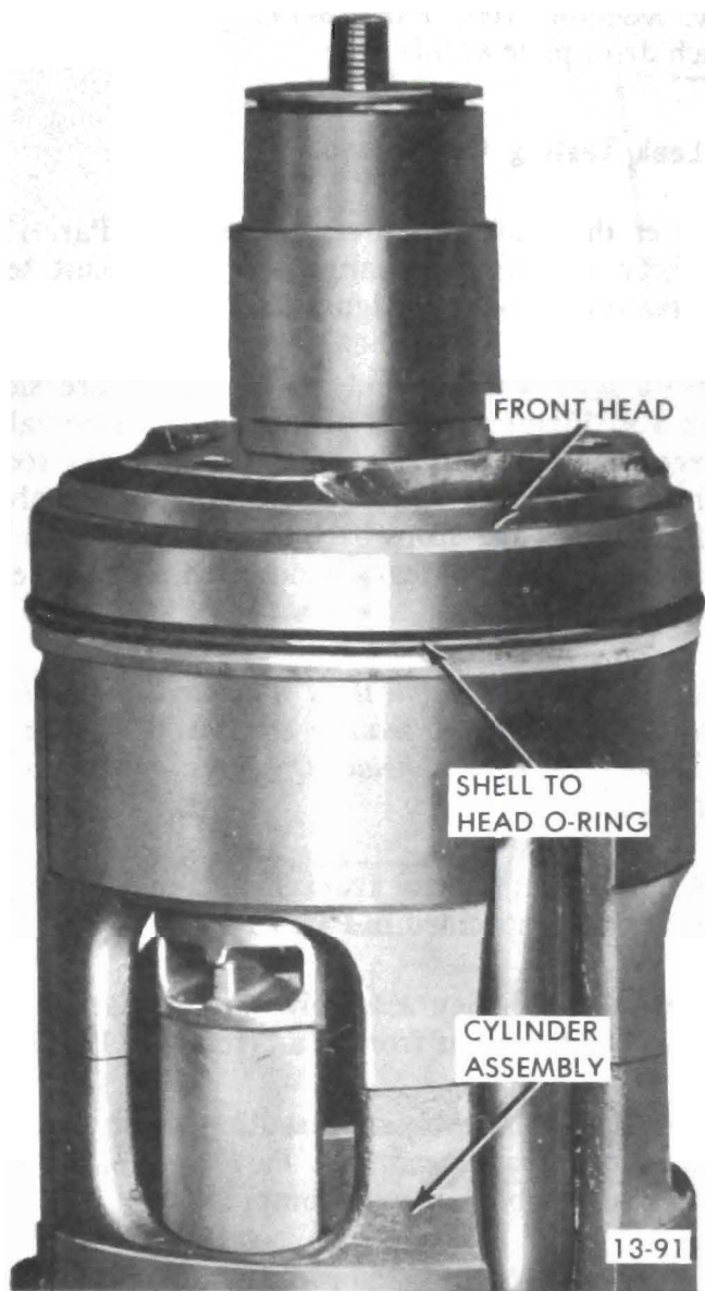
Figure 13-73 Shell to Front Head O Ring Installation
