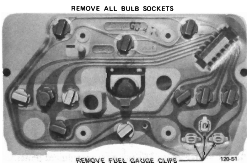
Figure 120-46 Replacing Printed Circuit
