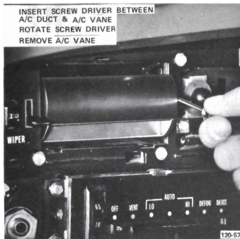
Figure 120-52 Removing A/C Outlet Vanes
