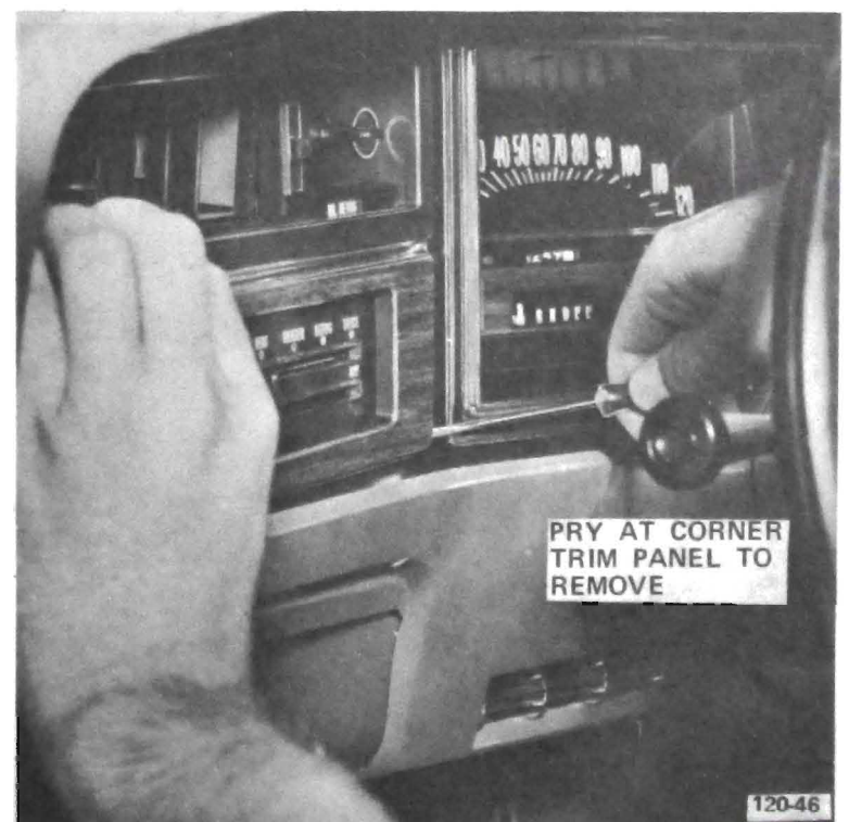
Figure 120-41 Removing Instrument Trim Panels
