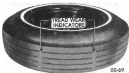
Figure 00-16 Tread Wear Indicators
