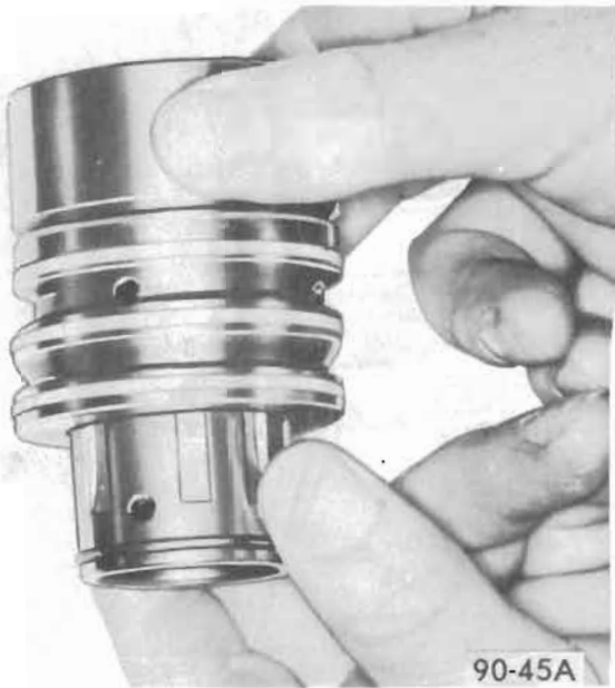
Figure 90-45 Removing Spool Valve
