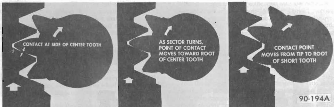
Figure 90-23 - Steering Gear Tooth Contact
