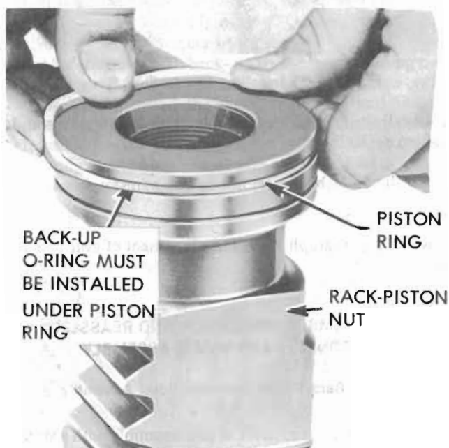
Figure 90-59 Installing Rack-Piston Ring on Rack-Piston Nut
