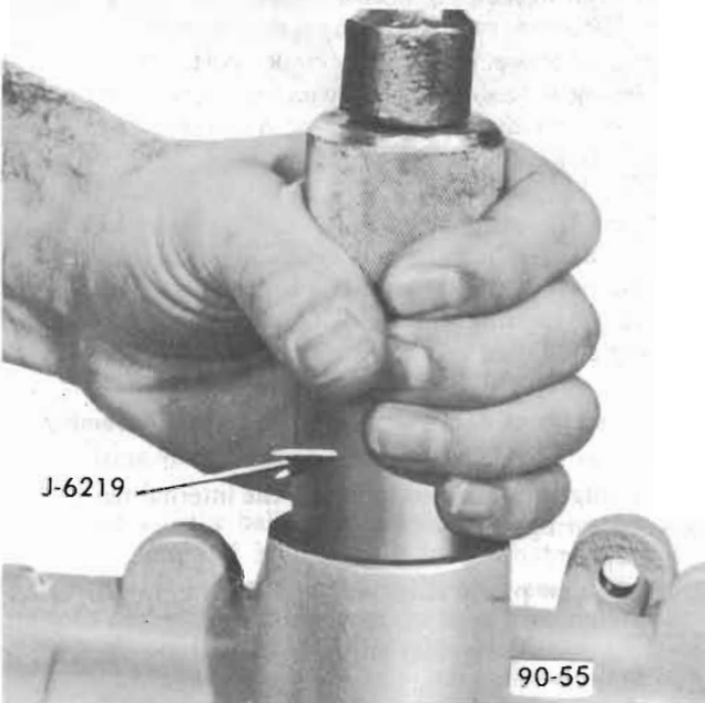
Figure 90-55 Installing Pitman Shaft Seals
