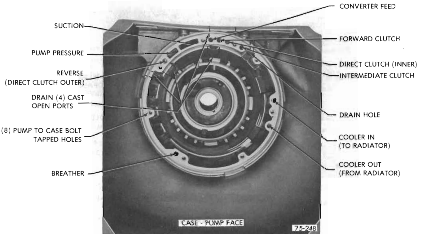
Figure 75-12 - Case - Pump Identification of Oil Channels
