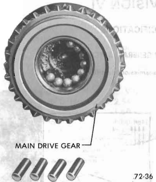
Figure 72-34 - Installing Needle Roller Bearings
