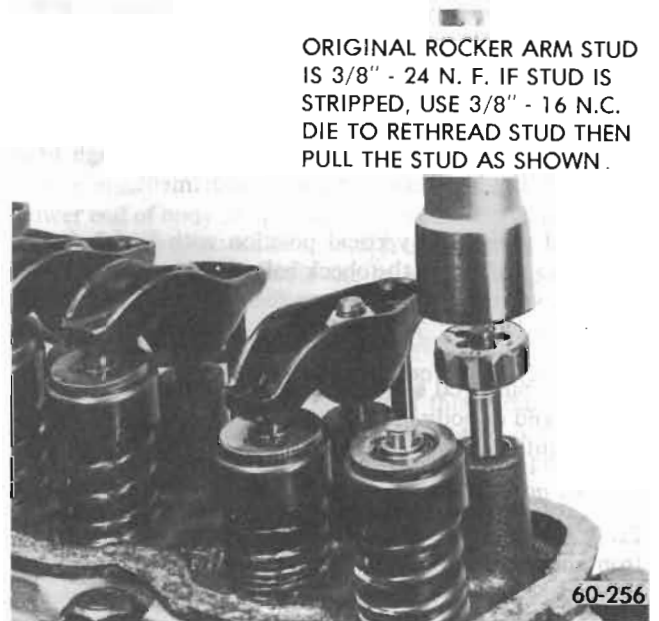
Figure 60-19 - Removing Stripped Rocker Arm Stud
