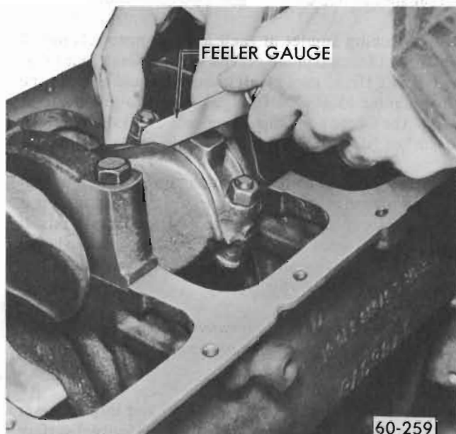
Figure 60-24 - Measuring Connecting Rod Side Clearance
