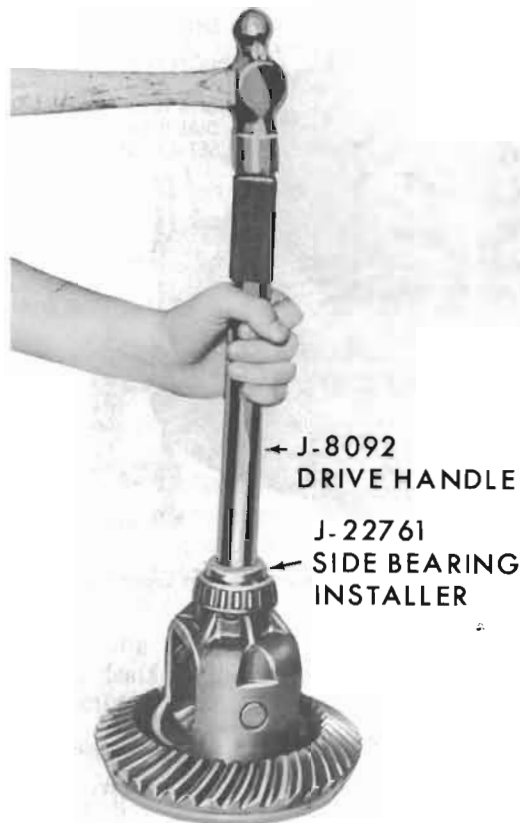
Figure 40-138 - Installing Differential Side Bearings
