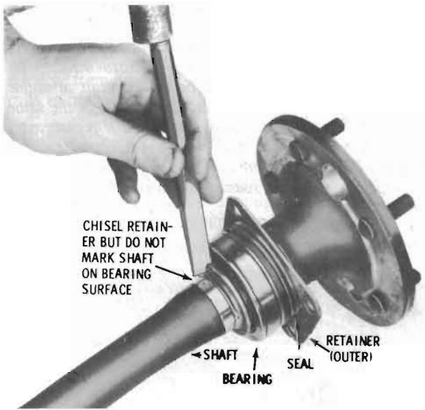
Figure 40-113 - Removing Axle Shaft Bearing Retainer
