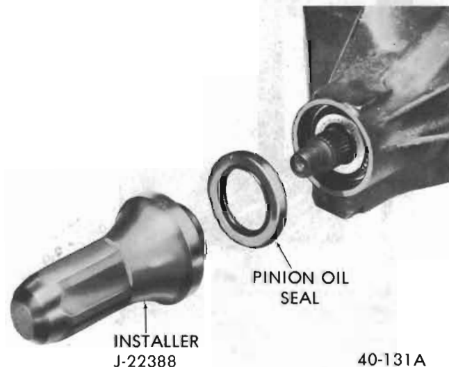
Figure 40-134 - Installing Pinion Oil Seal
