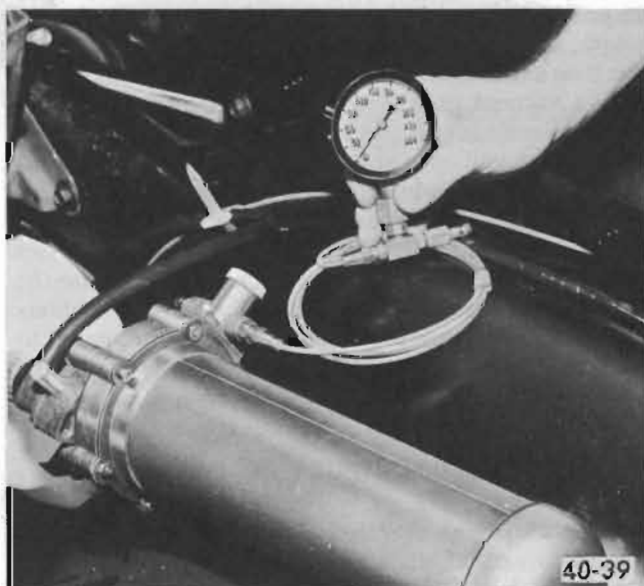
Figure 40-9 - Test Gage Installed on Regulator Valve
