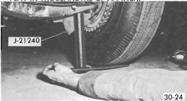
Figure 30-5 - Ball Joint Checking Gauge Installed
