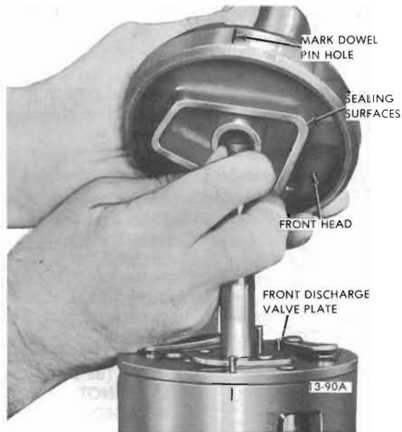
Figure 13-64 Placing Front Head on Cylinder Assembly
