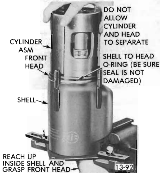
Figure 13-66 Installing Front Head and Cylinder Assembly in Shell
