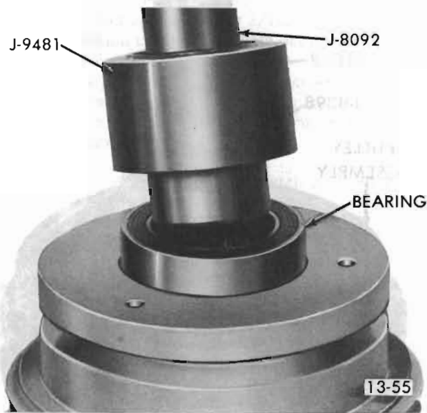
Figure 13-32 Installing Bearing into Pulley Assembly
