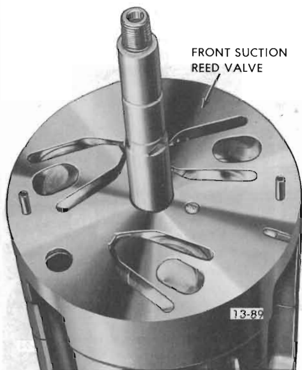
Figure 13-63 Front Suction Valve Reed Disc Installed
