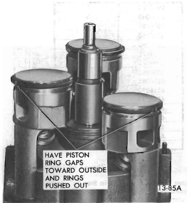
Figure 13-60 Pistons Positioned in Stair-Step Arrangement
