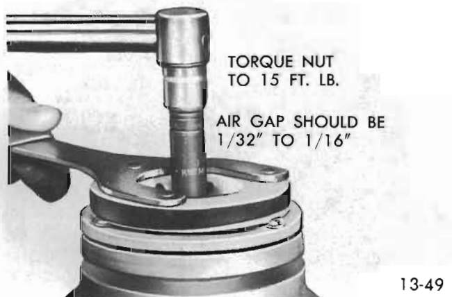
Figure 13-26 Torquing Shaft Nut
