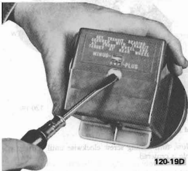
Figure 120-19D Adjusting Aimer to Compensate for Floor Slope
