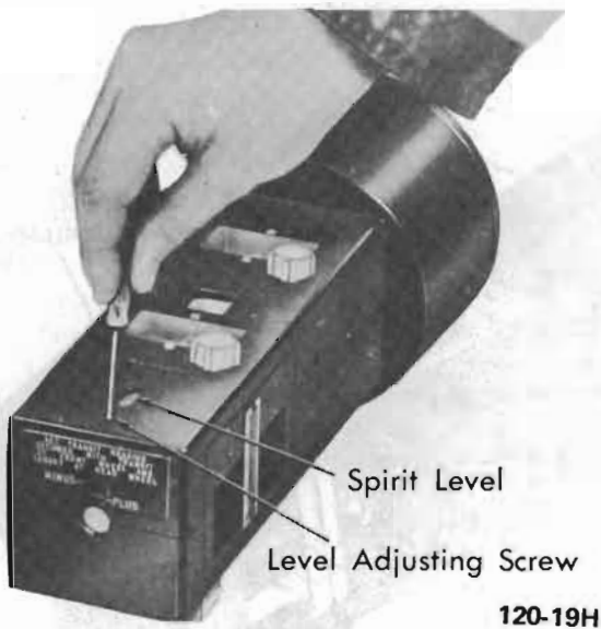
Figure 120-19H Adjusting Vertical Calibration
