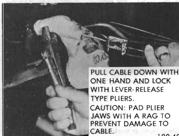
Figure 100-1 Using Parking Brake to Keep Rear Wheel From Rotating
