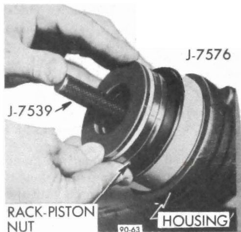
Figure 90-75 Installing Rack-Piston Nut - 46-48-49000 Series
