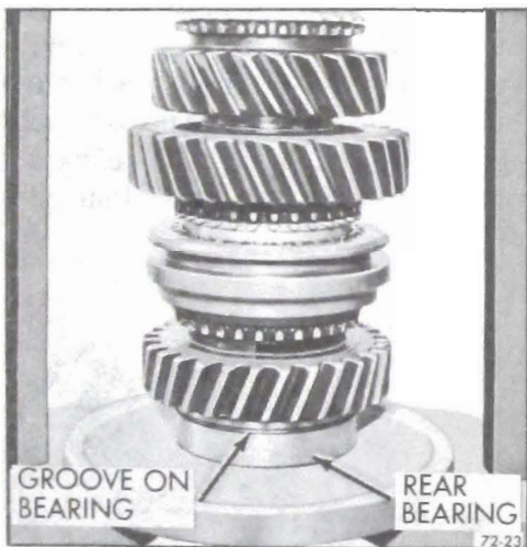
Figure 72-322 Installing Rear Bearing
