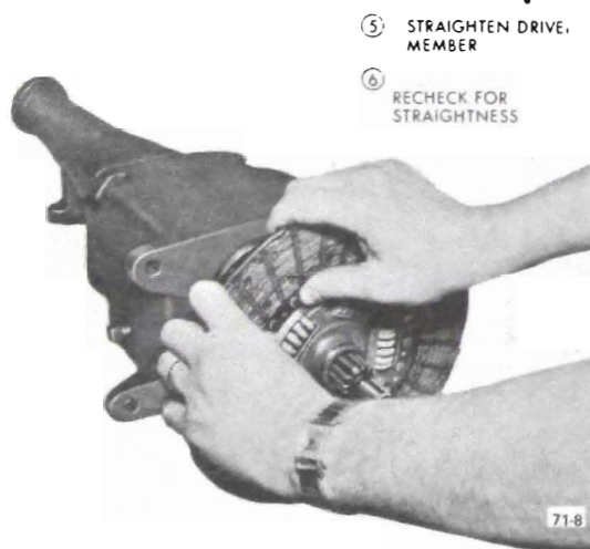
Figure 71-8 - Checking Driven Plate Run-Out
