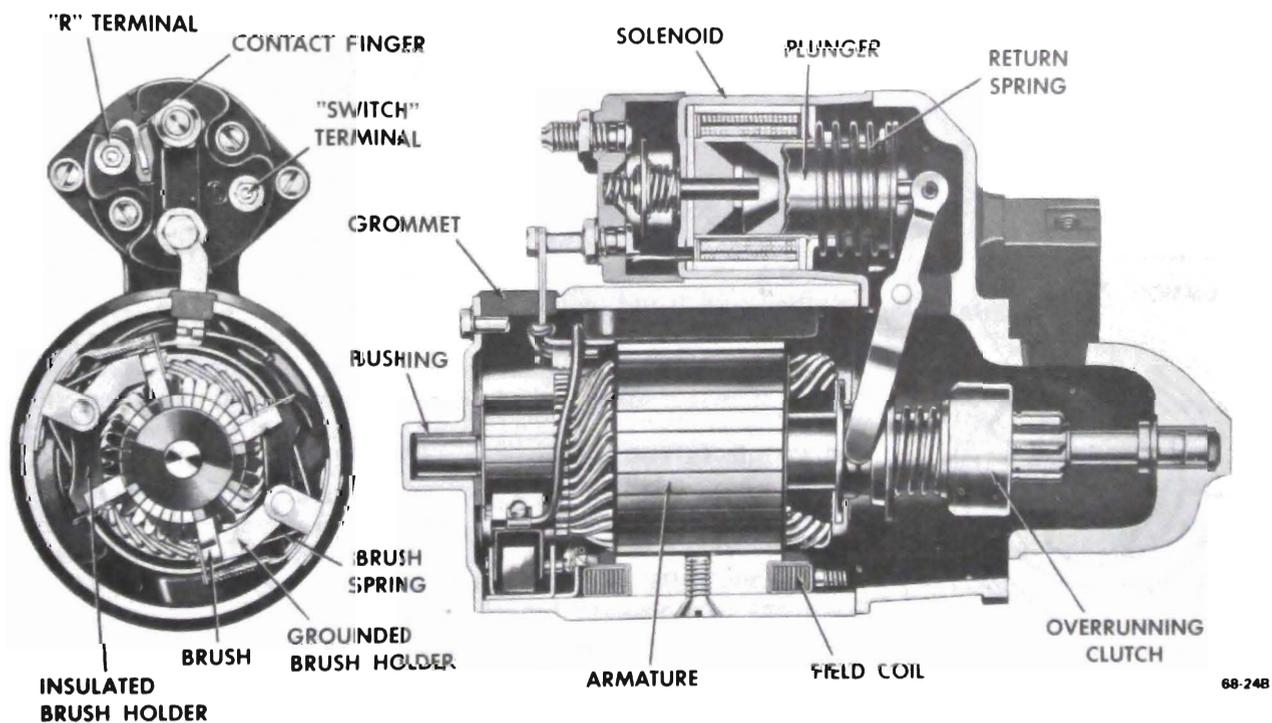
Figure 68-18--Starting Motor - 455 Engines
